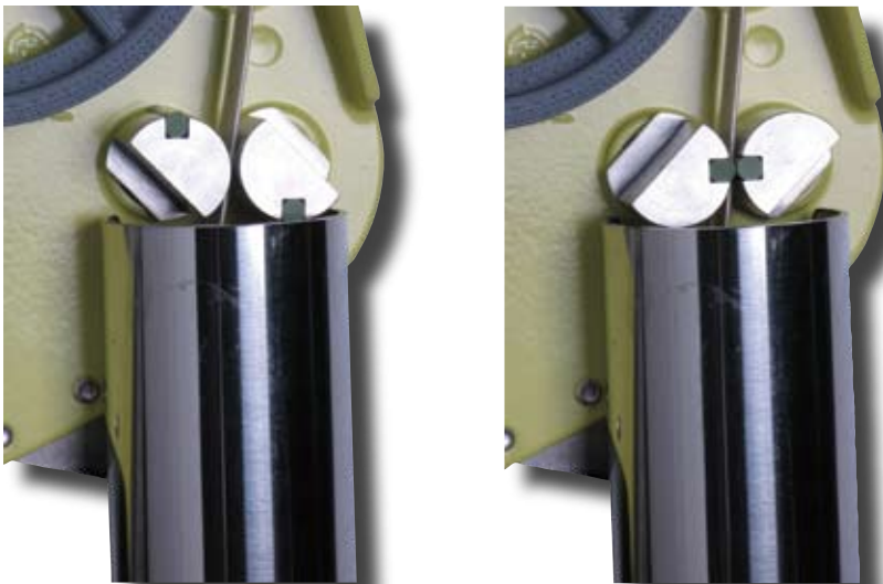
Protection tube to avoid spills and keep working space clean
